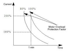
Fig.FA-1 Motor Overload Protection Factor
