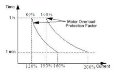
Fig. FA-2 Motor Overload Protection Factor Setting
