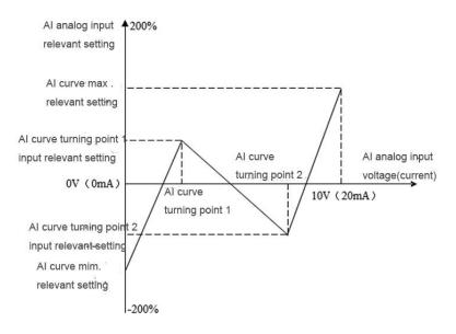
Figure F6-2 Almulti point curve diagram
