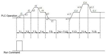
Fig.F9-2 Maintain Last Stage after Single Cycle
