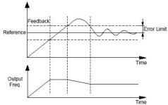
Fig. F8-3 Error Limit Schematic Diagram
