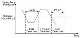
Fig. FA-4 Closed Loop Feedback Loss Detection
