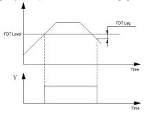
Fig.F7-8 Frequency Level Detecting
