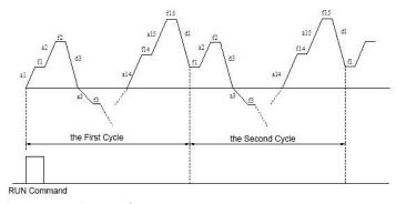
Fig.F9-3 PLC Continuous Cycle
