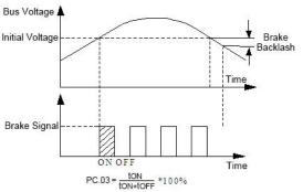
Fig. FC-1 Dynamic Braking
