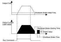
Fig. F1-4 Stop DC Braking
