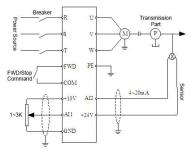
Fig. F8-1 Analog Feedback Control System
